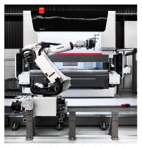
Fully automatic Bending Cell: The Bending Cell is as ideally suited for the processing of long job lists as for changing orders – from small batch sizes right through to large series.
