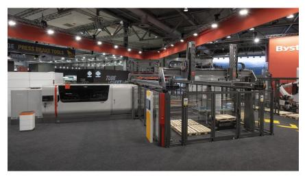
The Production Line is a fully automated manufacturing solution for the cutting, transporting, sorting, and storing of sheet metal parts. Solutions for the pre-processing of sheet metal parts can also be integrated.
