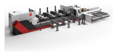
FL 170 3D: Wide spectrum of applications for the cutting of steel, stainless steel, aluminum, and non-ferrous metals in diameters from 12 to 168 millimeters and workpiece lengths up to 12.5 meters.
